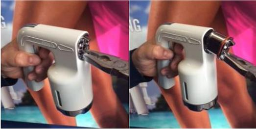
Using pliers, carefully remove the front by grasping the lower section & pulling straight out. Poke the air holes in that piece with a paper clip to free any debris.
