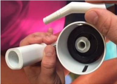
Gently wiggle out the pick-up tube so you don't move the bolt the tube is seated in (you may need those pliers if it is stuck in place). Poke out any gunk with a bent out paper clip or skewer in both the tube and the hole where it came from.
