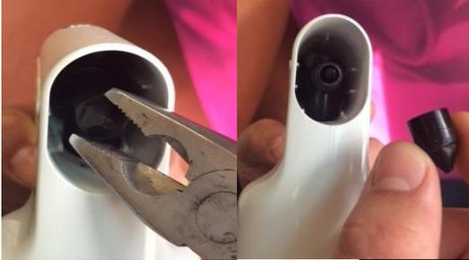
Using the pliers gently twist to the left to loosen the front black nozzle. You can then use your fingers to completely remove it.
