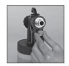
CAUTION DO NOT over tighten the screw as this will cause damage to the end of the spray needle.
